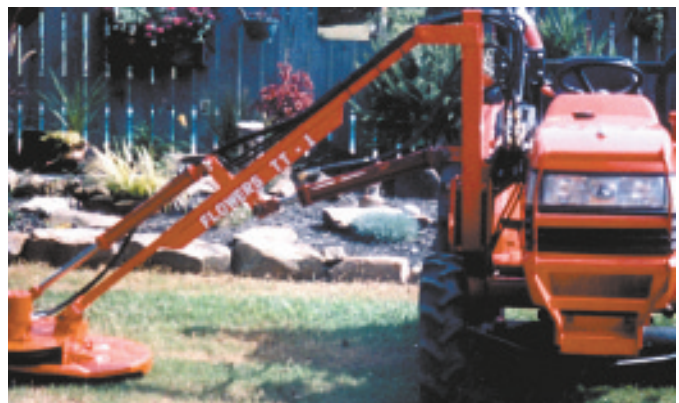
Side-mount mower extends about 7 ft. out from side of tractor. The arm it’s mounted on raises mower to 5 ft. above the ground or lowers it to 2 ft. below the tractor wheels.
