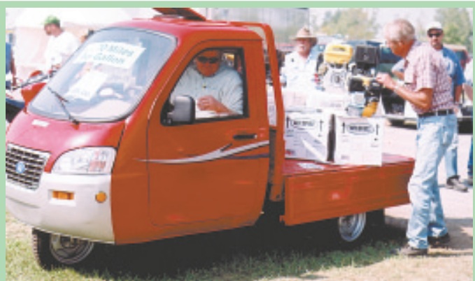
Chinese-made 2-passenger mini truck is powered by a 17 hp liquid-cooled engine with a 5-speed manual transmission. It has a single front wheel and sells for just $5,495.
