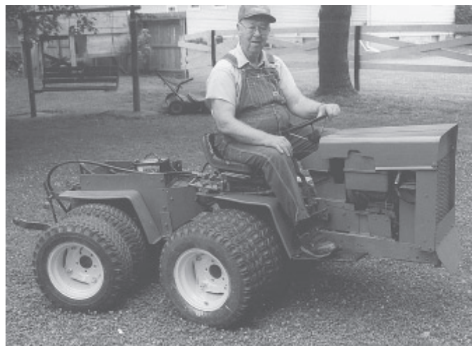
Milton Ruppert enjoyed the challenge of building this 4-WD articulated garden tractor out of a pair of salvaged Cub Cadet garden tractors.
