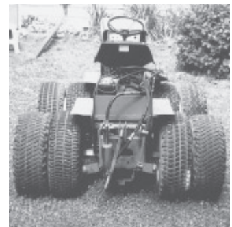
Dual-wheeled tractor is equipped with a 3-pt. hitch and hydraulic steering system.
