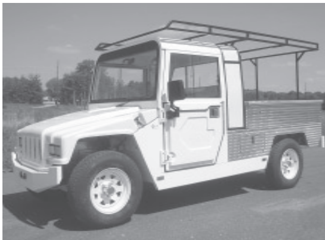
Two-passenger truck has a maximum range of 55 miles between charges and can reach a maximum speed of 25 mph.
