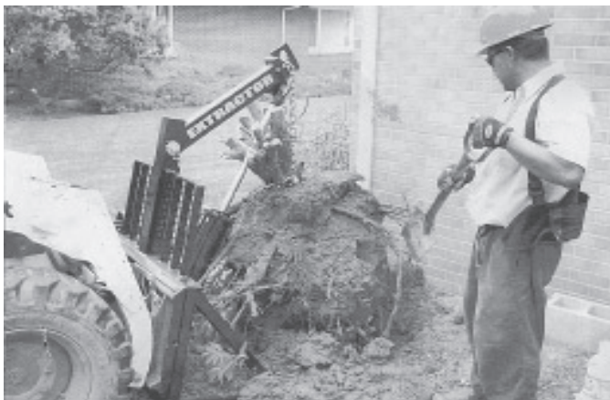
Skid steer "Extractor" lets you pull up close to a building and exert up to 15,000 lbs. of vertical force. All the leverage is against the ground, not against the machine.
