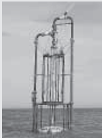
Wave-driven Seadog pumps are designed to power electrical generators.
