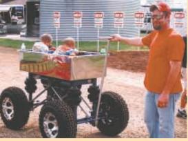
**Bill Cates** made this sporty wagon out of truck and golf car parts. The 4 by 2-ft. box is fitted with air bags off a semi tractor.
