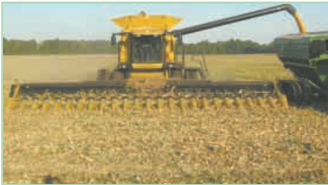
At 40 ft. wide, new Geringhoff Northstar header can harvest 24 20-in. rows at a time.
