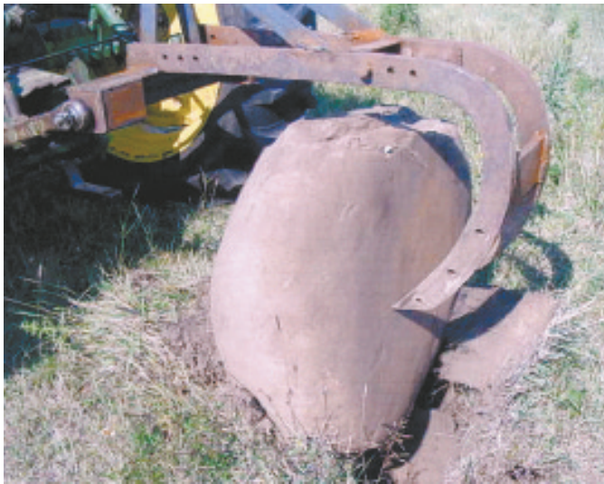
Ken Lake has been making 3-pt. mounted stone plows for several years. "In the spring when the ground is soft, the boulders just pop right out," he says.
