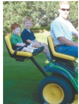
Terry Martin made a double safety seat with seat belts so his kids can ride with him while he mows his yard.
