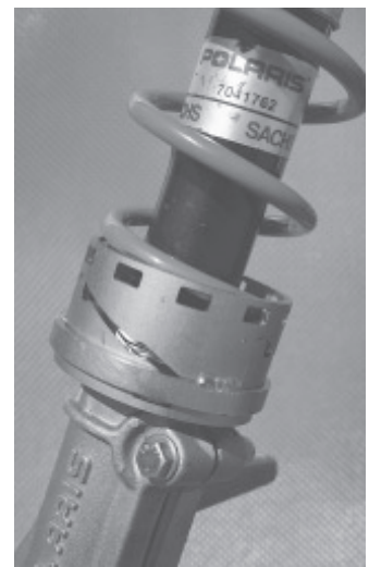
Pre-Gressor kit installs on ATV's front suspension forks. It can be quickly adjusted as needed to handle heavier loads.
