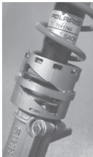
Pre-Gressor kit installs on ATV's front suspension forks. It can be quickly adjusted as needed to handle heavier loads.
