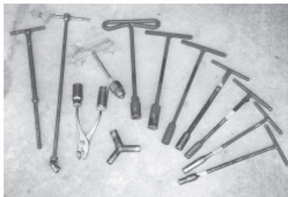
David Novotny welded steel rod and rebar into deep well sockets to form handles about 1 ft. long, with a 5-in. long cross "T" at one end.
