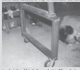
ing height of hisA-frame hoist. His solution was to build two rectangular frames and weld them onto each side of the A-frame, adding a pair of caster wheels on each side. The frames added an extra 3 ft. of height.
