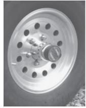
Battery-powered, digital counter notes every revolution the tire makes, calculating miles or kilometers traveled.
