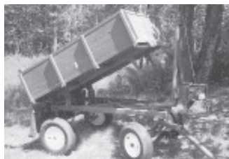
Winch-operated dump wagon is equipped with a “flip flop” tailgate to empty loads.
