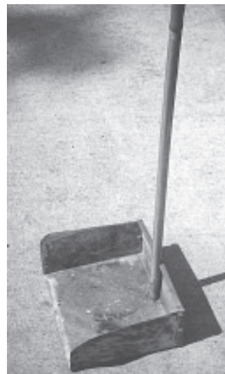
Bill Reeks extended the handles on a pair of hand shears (left) for trimming grass around trees and buildings. He also added an extended handle to a dust pan in his shop.
