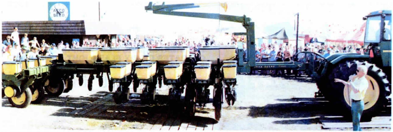
New Deere planter toolbar pulls from the tractor's 3 pt. hitch in both the field and road position.
