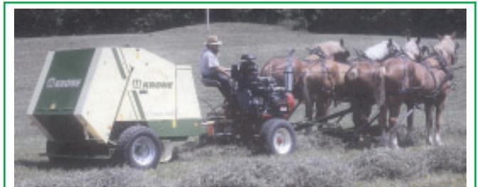
Engine-powered forecart provides all the pto power needed to pull a Krone round baler.
