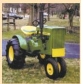
Kit is designed to convert tractor to a narrow front end and comes with a pedestal and steering rod, as well as oversize front and rear wheels.
