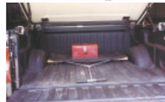
"Cargo shuttle" rides on rollers. T-shaped handle pulls it back for easy loading.
