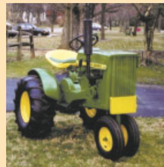
Kit is designed to convert tractor to a narrow front end and comes with a pedestal and steering rod, as well as oversize front and rear wheels.
