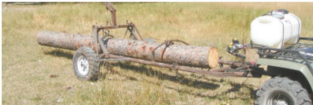
Two-wheeled, winch-operated log hauler is designed so that as log is lifted, the top front end of it comes into contact with a stationary bar, which lifts rear end of log off the ground.
