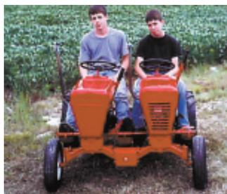
Derek and Trent Barger built this side-by-side tractor out of a pair of old Wheelhorse garden tractors.
