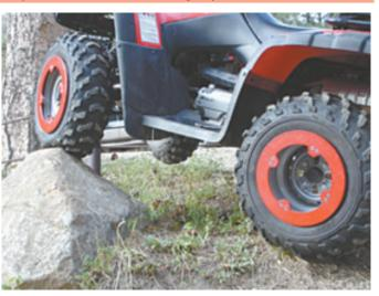
Wheel-mounted poly rings are designed to prevent damage to ATV's wheel rims. Rings extend about 1/2 in. above the rim to protect bead area of tire.
