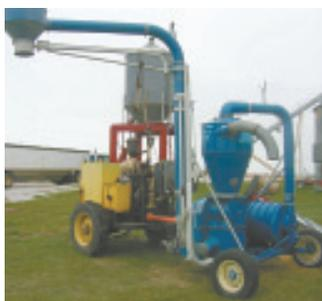
**"It's only 8 ft. long so it'll fit into tight spots," says Tom Peterson about the self-propelled grain vac he made out of irrigation parts.**
