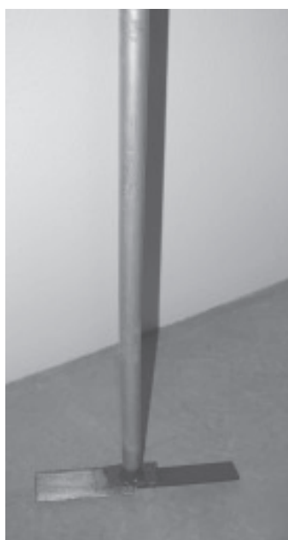
Power mixer is designed to be operated by a drill. Starting the drill opens up paddles to a 15-in. diameter. The paddles grind up material as they rotate and collapse when drill is turned off.
