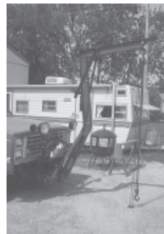
Brad Hurst Sr. designed this hoist to fit his snowplow truck. It will lift up to 1,000 lbs. and comes in handy for doing mechanical work on small pickups and lawn mowers.
