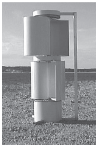
Self-governing cylindrical windmill keeps producing energy when other windmills have to shut down due to high winds. Photos show windmill open (left) and closed.
