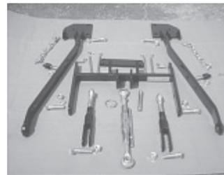
Cat. I 3-pt. hitch is designed to bolt onto a number of Deere lawn and garden tractors.
