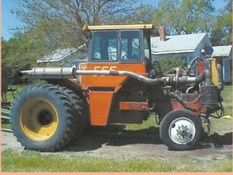
Dan McAmoil replaced the engine and transmission on his Versatile 555 2-WD articulated tractor with a 325 hp Cummins diesel engine out of a Freightliner semi tractor.
