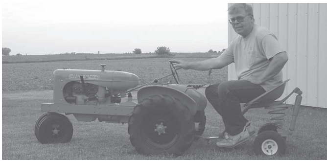
To operate the tractors, he made a small two-wheel cart with a tractor seat on it that hooks to the drawbar and pulls him around.
