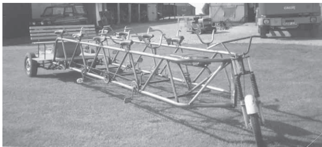
One-of-a-kind 12-passenger bike has eight sets of pedals and a wooden bench seat on back for three passengers.
