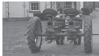
Rear wheels are 7 1/2 ft. apart which allows dual tractor to be easily transported over the road.
