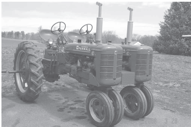
David Evans put together this pair of Farmall C tractors, welding the spider gears together so gears can be shifted from either tractor.
