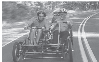
Human-powered car is designed to be powered by four people, each pushing and pulling on their own T-bars.
