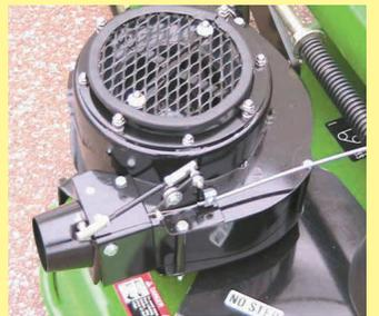
Add-on string trimmer (left) sucks grass up into trimmer lines. Blower fits on same mounting bracket that mower-trimmer fits on and is also belt-driven.
