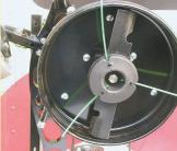
Add-on string trimmer (left) sucks grass up into trimmer lines. Blower fits on same mounting bracket that mower-trimmer fits on and is also belt-driven
