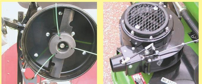
Add-on string trimmer (left) sucks grass up into trimmer lines. Blower fits on same mounting bracket that mower-trimmer fits on and is also belt-driven.
