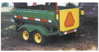
"It looks nice and pulls easy behind a pickup, 4-wheeler, or garden tractor," says James Stump about the trailer he made from a 275-gal, fuel oil tank. Trailer has a removable gate on back, and a small toolbox and also a jackstand on front
