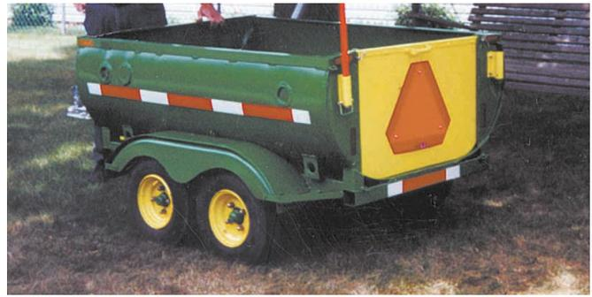
"It looks nice and pulls easy behind a pickup, 4-wheeler, or garden tractor," says James Stump about the trailer he made from a 275-gal. fuel oil tank. Trailer has a removable gate on back, and a small toolbox and also a jackstand on front.
