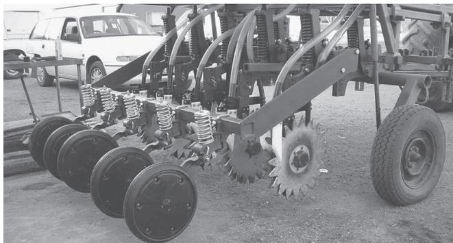
StubbleStar row opener uses star-shaped discs. It's able to operate in thick residue that can be left in place to suppress weeds.
