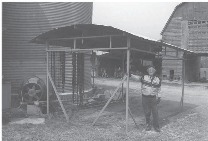
Hubert Smith used sections of a damaged 3,000-bu. bin to make this car port. It measures 12 ft. wide by 22 ft. long and mounts on steel runners.
