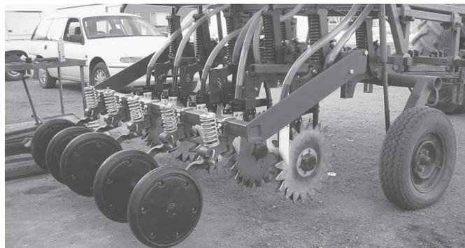
StubbleStar row opener uses star-shaped discs. It's able to operate in thick residue that can be left in place to suppress weeds.
