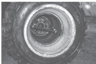
A 6-in. metal spacer between wheel rims keeps wheels from clogging up with mud. A wrench.
