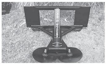
Tree shearer slices through trees up to 3 in. in diameter. Cutting assembly consists of two 14-in. dia., overlapping discs that are smooth with one beveled edge.
