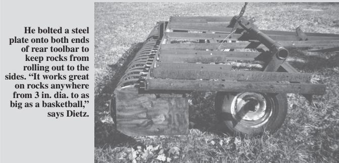
He bolted a steel plate onto both ends of rear toolbar to keep rocks from rolling out to the sides. "It works great on rocks anywhere from 3 in. dia. to as big as a basketball," says Dietz.
