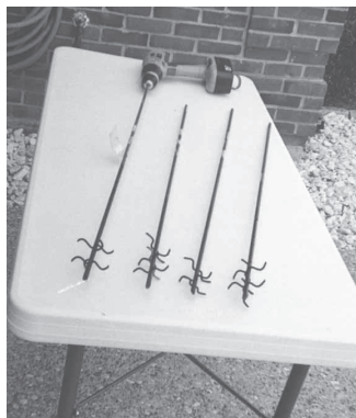
Equipped with hardened steel tines, the 33-in. long steel tool fits into any variable speed electric or cordless drill.
