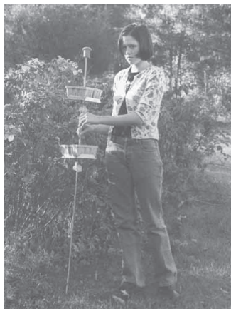
Stick lets you pick berries with both hands. Just stick pole in the ground and put basket on pole-mounted plate.
