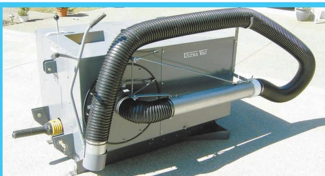
UltraVac uses a big 22-in. impeller connected to a 16-ft. long flexible rubber hose.
