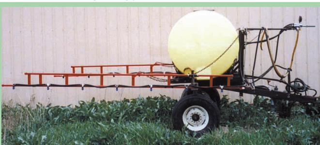
John Rathjen built this 32-ft. boom from two parallel pipes spaced 6 in. apart.
