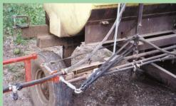
loaded folding mechanisms, one on each nism on boom centered. To fold boom back, Rathjen unhooks side. Rathjen sawed off the front three straps. Clevis with pin holds boom in transport.
