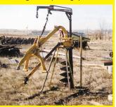
apart, with two 32-in. lengths of sq. tubing welded between them. A 7-ft. 2-in. high length of tubing is welded upright at the center of the 32-in. piece. A 42-in. length of tubing is welded at a right angle to the top of the upright and supports a hook with a turnbuckle attached to it.
