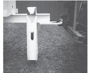
When parked, two V-notches on top of hitch stand hook it into place.
