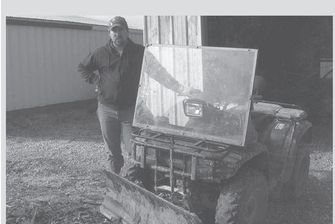
Add-on windshield is held in place by a steel frame that bolts to the front rack.
