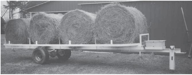
What makes Martin's 30-ft. trailer unique is that he can hitch and unhitch quickly without getting off the tractor.
