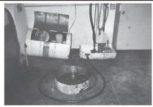
An electric-powered gear pump sucks oil from a portable oil pan into a 55-gal, storage drum.
