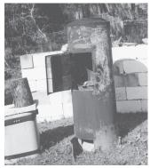
Furnace is made out of an old water tank lined with firebrick. Ferreira uses furnace to melt down cast aluminum lawn mower motors and other cast parts.
