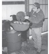
Connecting an old tractor oil pan to a barrel makes it easy to dump used oil, says Mike Miller.
