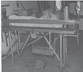
drill, mounted at one end, drives a 1-in. threaded rod one way and then the other. I use a foot switch on the floor to hold the metal with both hands. A chain drive connects the two 1-in. threaded rods at each end so that it opens and closes evenly. The brake is also hinged to the shop wall at one end, allowing me to roll it out of the way whenever it's not needed."
