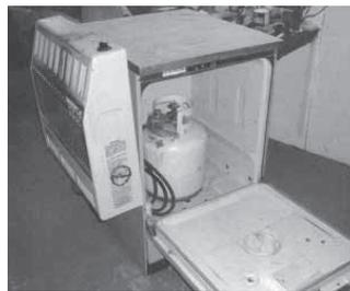
the heater. The door locks and seals the tank inside. It can be easily moved anywhere in the shop I need heat. The top also works as a portable stand for my drill press, wood planer, etc."
