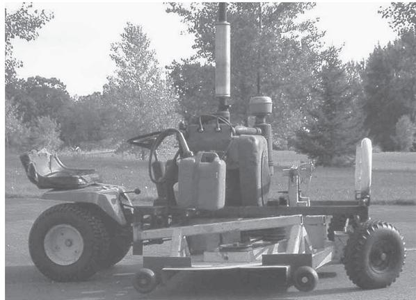
**Tony Hargreaves cut a Simplicity garden tractor in two and mounted a big Wisconsin engine and deck mower between the front and rear ends.**
