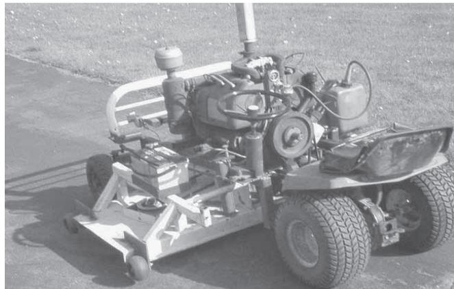
**The mower deck has three 25-in. blades that overlap slightly to give it a 72-in. cut. The center blade spindle has a four-belt pulley on it.**
