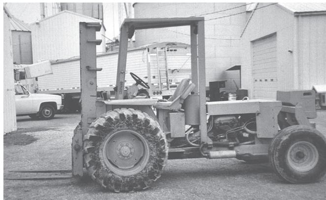
**Koehler's home-built forklift is equipped with a 10,000-lb. mast and rides on tractor-size tires. "We use it a lot, for everything from moving bulk seed to hauling logs to our wood splitter."**
