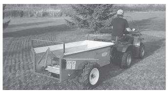
"Unlike other small manure spreaders on the market, you don't have to get off the machine to engage this spreader. The lever is right behind the seat," says Tom Roth, owner of Roth Manufacturing.
