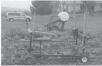
To steer the rig, Brown took the steering mechanism off an old garden tractor and adapted it to fit the front of the frame.
