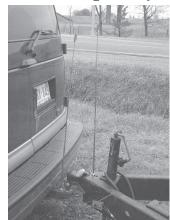
Simple magnetic hitch guides stick to ball hitch and trailer tongue.
