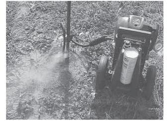
Two-wheeled Skeet-Daddle is powered by a 4-cycle Honda engine and weighs 20 lbs. No mixing of chemicals is required. You just insert a can of Resmethrin.
