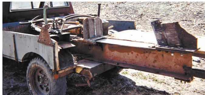
Splitter's hydraulic pump is powered off the pickup's rear driveshaft.
