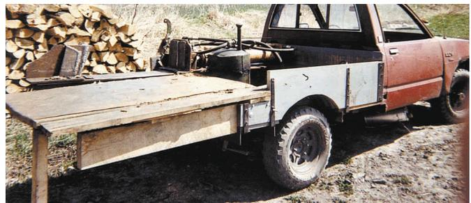
Walter Fifelski uses an old rusted out Chevy 4-WD pickup to power this log splitter.
