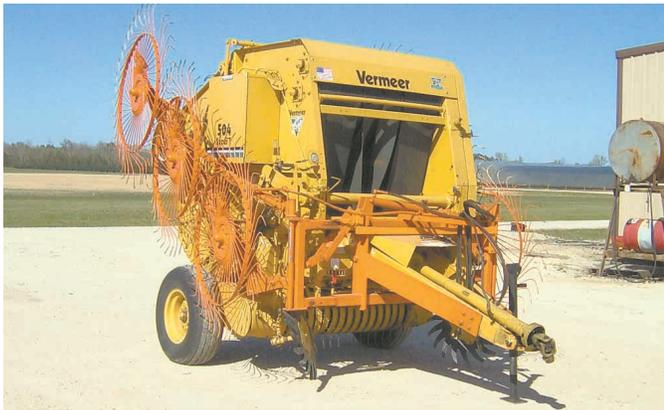
Baler-mounted rake eliminates the need for a separate raking operation in the field.
