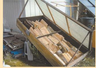
Plywood box has a corrugated fiberglass lid set at a 30-degree angle. Temperature inside dryer can reach 160 degrees, enough to quickly dry firewood.
