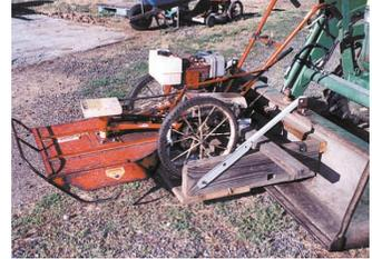
DR brush mower attaches to front-end loader, which is lifted up to cut.
