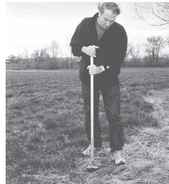
"Bait stick" tube has a spring-loaded base. It meters out bait as base is pushed against a hole.
