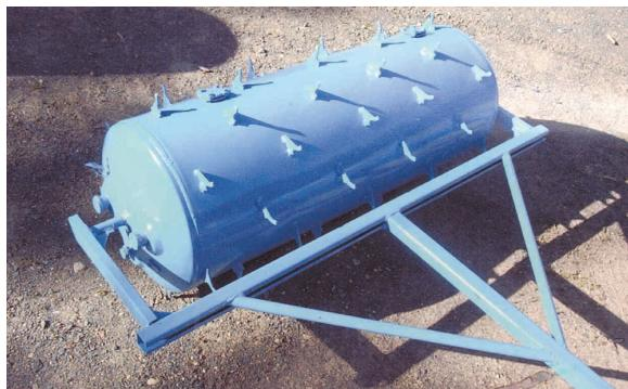
Aerator was built by welding teeth to an old 50-gal. water heater tank.
