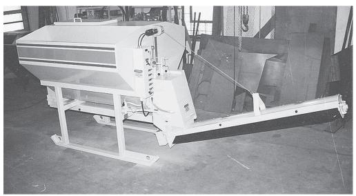
Luoma's 3-cubic yard mixer combines sand, cement and water in an auger tube fitted with specially-designed paddles.
