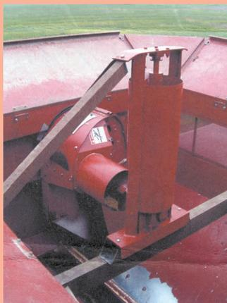
**"Bubble up" auger was made by replacing the original cross fill auger with an auger that just goes to the center of bin. There, it fastens to a right angle gearbox which then drives another auger that goes straight up.**
