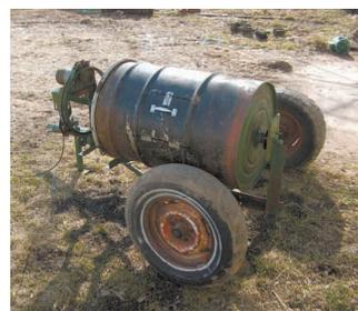
**Using a jig saw, he cut a 12-in. wide door into side of drum.**
