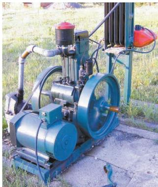
**With a simple design, heavy flywheel and low rpm's, the Lister engine will far outlast newer, high rpm engines, says George Breckenridge, who sells Lister engines.**
