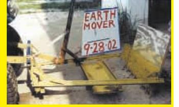
has a scarifier on back, and a skid plate in the middle to keep the blade from going too deep.
