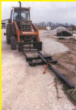
I needed a boom to lift rafters while building an extension onto my farm shop, so I built this unit that attaches neatly to a two-tine hoist on my front-end loader. The tines slide into square tubing on the boom. A short chain cinches the two pieces together, making them function as a unit. (Dan Neuman, 9800 Mansion Rd., Loami, Ill. 62661 ph 217 624-2200)
