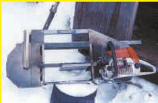
I use a Stihl 036 chain saw on an old Better Built band saw rig to cut logs into boards. The chain saw simply cuts in place of the band saw blade.
